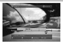
As a result of the high data transfer speed of the HDD, it is possible to play back recordings from the time shift buffer while the recording is still in process.
